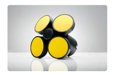
The Signature 250 ADCP is a medium-range current profiler with a suite of extra features. It has a current profiling range of 200 m, and can measure wave height, period and direction at depths as great as 150 m. The Signature 250 ADCP can also measure acoustic ranging to ice. Its compact design and low power consumption make it an ideal tool for long-term deployments in all waters.
