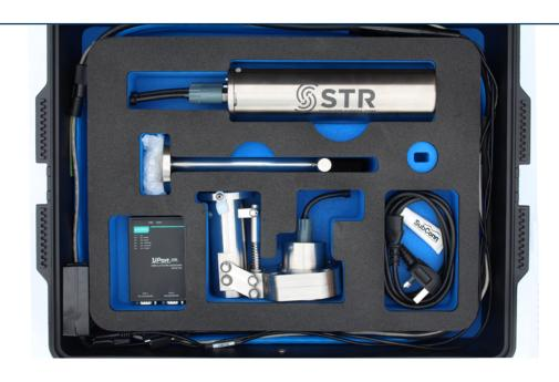
The STR SeaSonic Acoustic Flooded Member Detection System is a bespoke development providing the optimal accuracy and reliability attainable for acoustic flooded member detection. The system draws from experiences gained with the field proven STR SeaGamma FMD system. Unlike the STR SeaGamma system the STR SeaSonic system does not require the use of ionising radiation, this aids safety and transportation.
