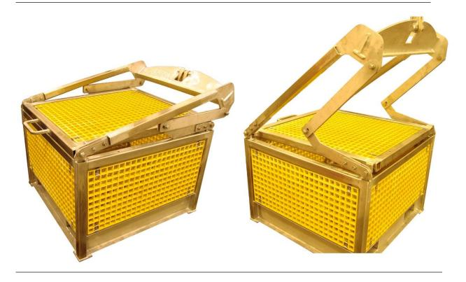
The IKM Subsea **Subsea Mini Basket** is designed for subsea lifting of tools and equipment. It is a lightweight structure made out of stainless steel and grating. Foldable lifting yoke for easy access during loading and unloading. The lid is locked when the yoke is in a lifting position, and can be removed if required.
